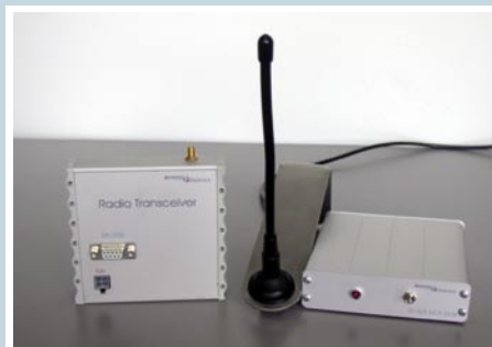
Above: Data transmission to PCMCIA-Data Logger or via Radio Module
